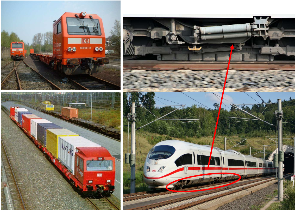
Figure 100: Powered container wagons 63
