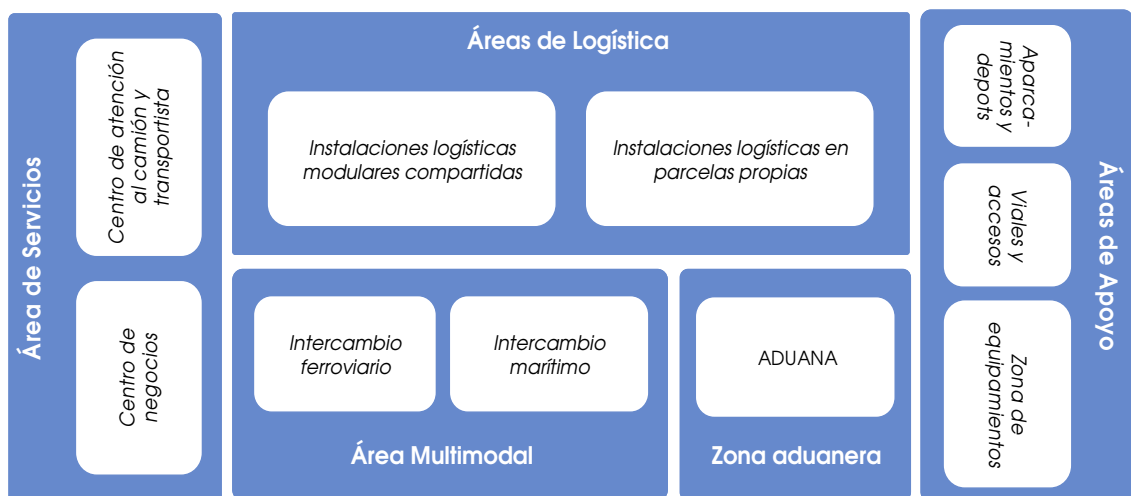
Figure 121: Functional layout of a standard logistic platform 75
