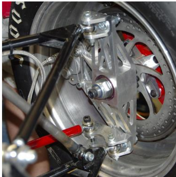
Figura 26. Manga de Eixo de um Fórmula SAE. Fonte: https://www.formulastudent.de/fsg/pr/news/details/article/pats-seven-deadly-sins-of-fs-design/
