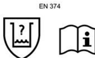
Figure 2 — Chemical pictogram for waterproof gloves and low chemical protection
