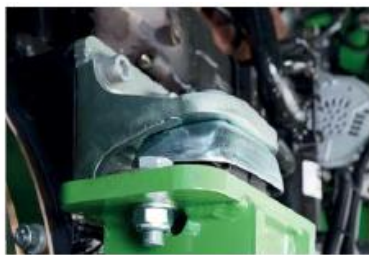
Low-vibration engine mounting reduces wear on components and lowers sound levels.
