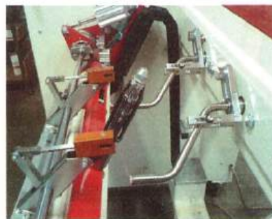
Yarn cutter with automatic release of yarn ends device
