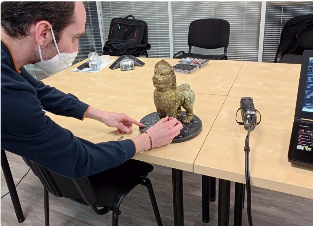
Our partner placing a few adhesive markers before a scan. Source: Aniwaa
