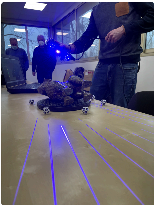
The SIMSCAN projects blue laser lines to calculate an object's shape in 3D. Source: Aniwaa
