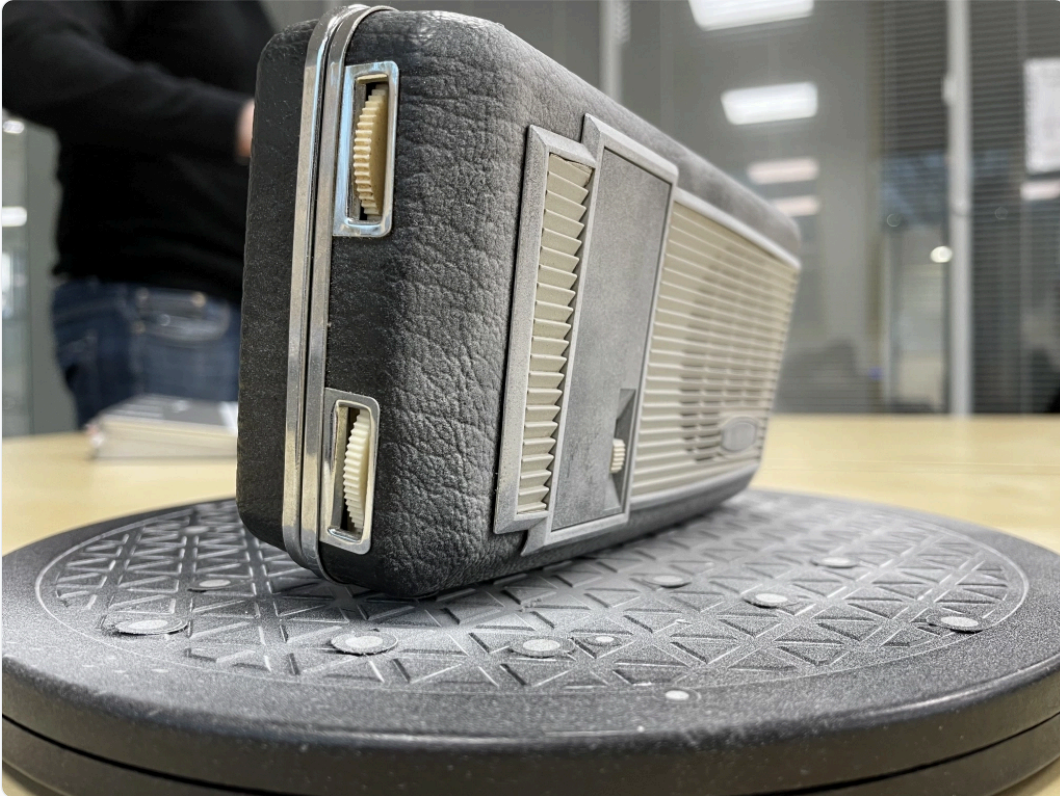
The transistor radio (upside down, as we had already captured the top part at this point) sprayed with AESUB Blue vanishing powder. Source: Aniwaa
