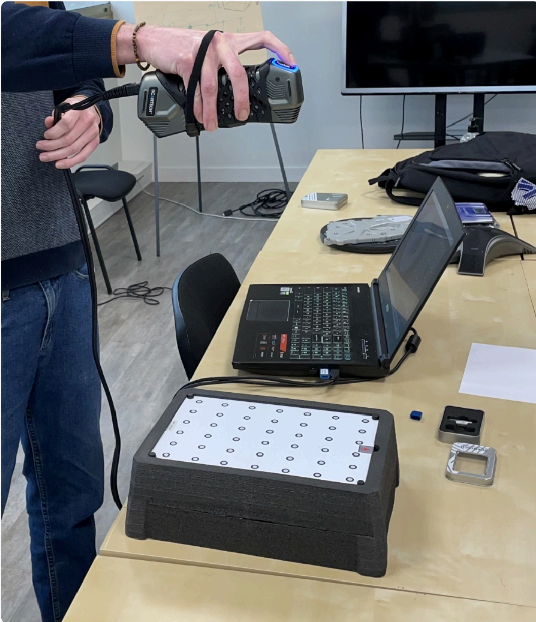
The calibration plate, glued to a block of foam. Source: Aniwaa
