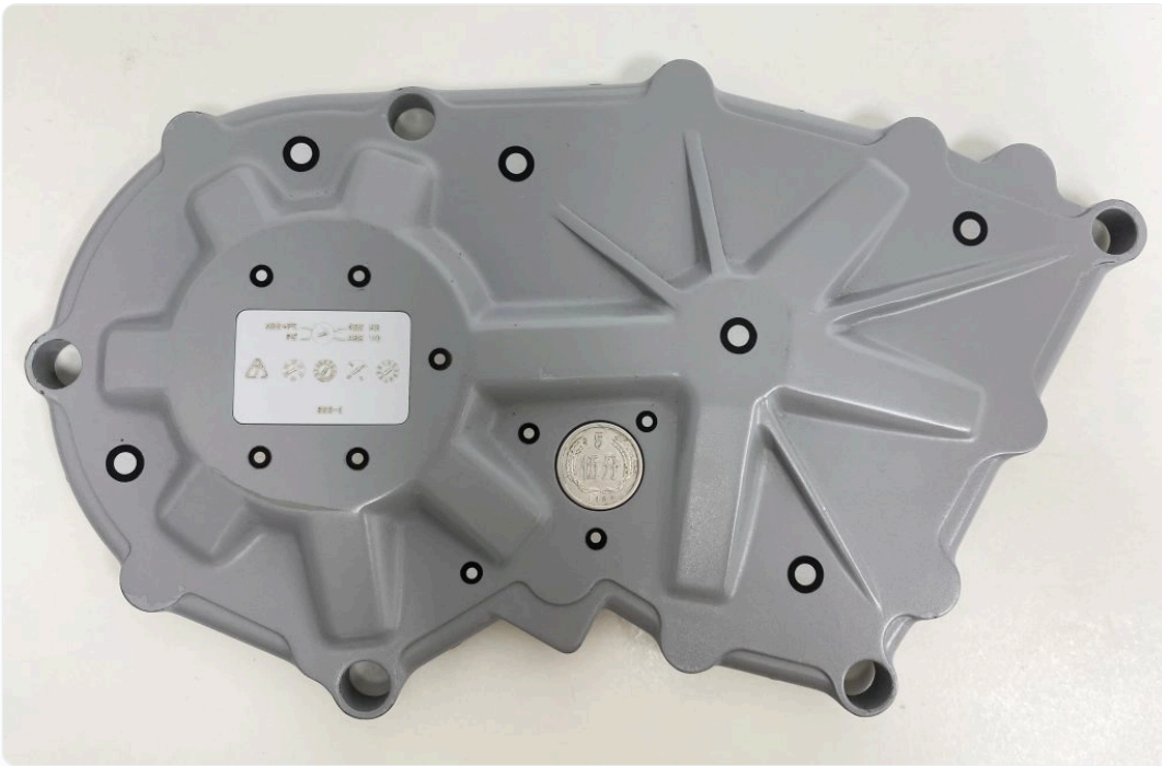
Closeup of the demo part. The light grey area to the left and the coin on the right feature very small and complex details. Source: Scantech
