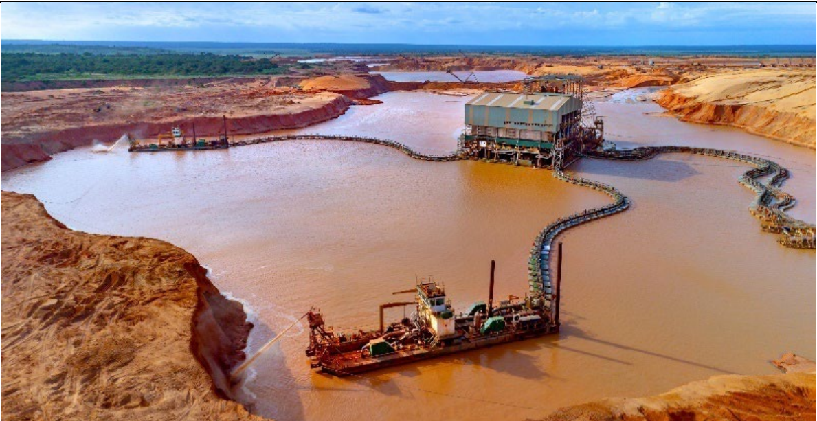
Figure 19: Floating Mining and Concentration Unit for Mineral Sands, Mozambique
