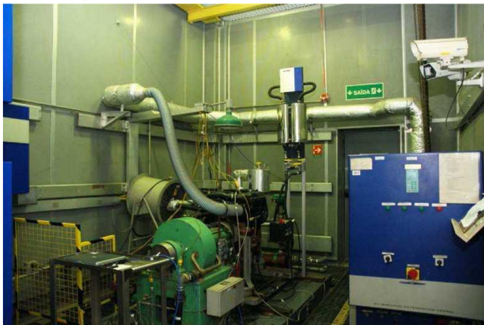
Figure 34 - Engine installed in CENPES's test bench.
