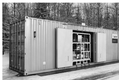
Figure 4. Chemical synthesis unit of the Soletair project with Ineratec's FT reactor (Copyright by Ineratec/VTT).
