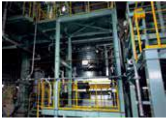
Plasma melting furnace
