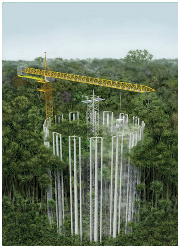
Figure 17: Laboratory in the forest. Structure for enrichment of CO 2 in the atmosphere
