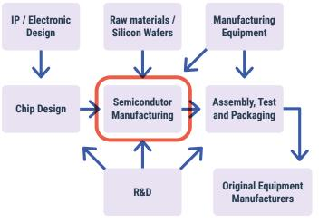
rall manufacturing process of the semiconductor wafers. The average time to fabricate finished semiconductor wafers, known as the cycle time, can take up to 14-20 weeks to complete for advanced processes.
