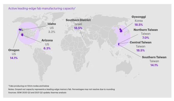
\*Schematic 3: Semiconductor Fabs producing on 10nm nodes
