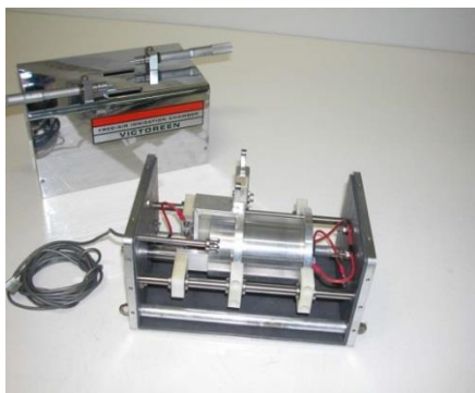
Figure I.6: Victoreen Free air ionization chamber, model 481[8].
