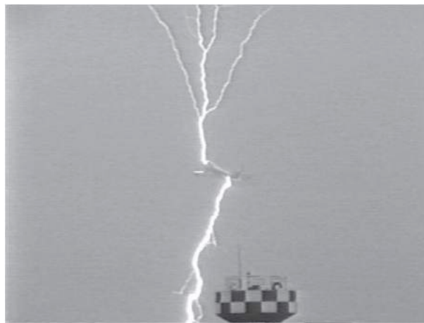
Figure 2.5 – Bidirectional leader development in an airplane struck by lightning.
