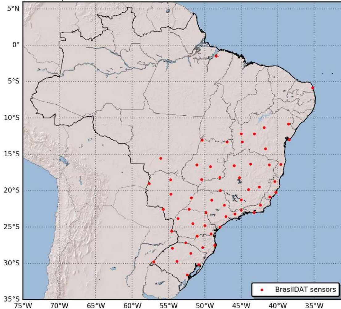
Figure 2.12 – Spatial distribution of the BrasilDAT sensors. Currently, the network operates with 60 sensors in 13 different states.
