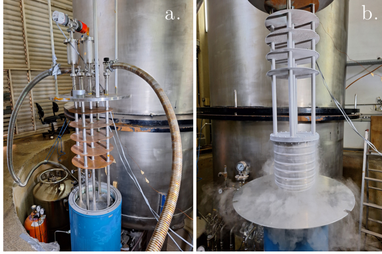
Figure a. shows the experiment run in its beginning, while diving in the dewar in the liquid nitrogen bath. Figure b. shows the dewar completely out the LN2, when the run was over.
