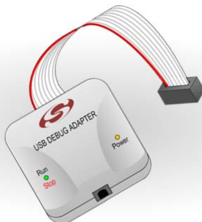
Figure 1. 8-Bit USB Debug Adapter
