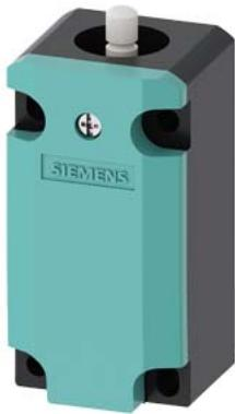
Basic switch for position switch 3SE51 Metal enclosure, according to EN 50041 Device connection 1 x (M20 x 1.5) 1 NO/2 NC quick action contacts without actuator head
