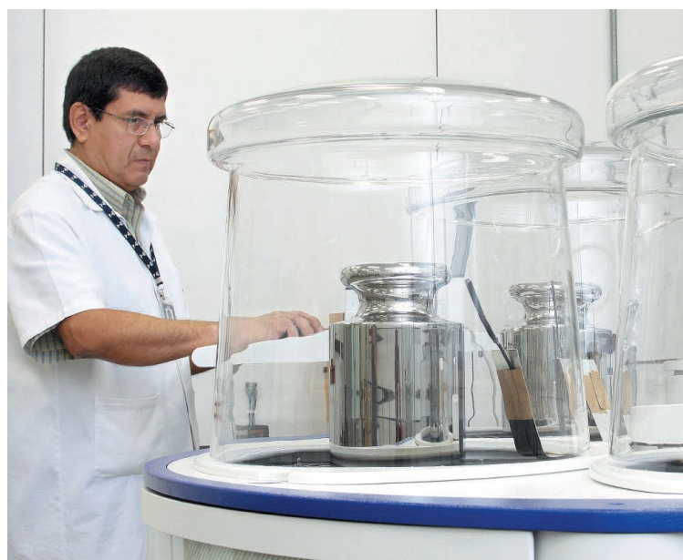
64-kilo mass comparison scales, resolution 0.1 mg
