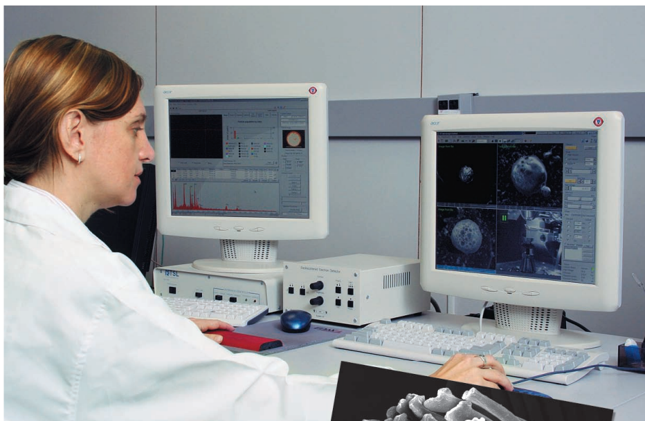
The Quanta 200 electronic scanning microscope set up in Inmetro's Material Metrology Division, which has been modernized to meet requirements for Forensic Metrology. In the photo, gunshot residues are being analyzed.
