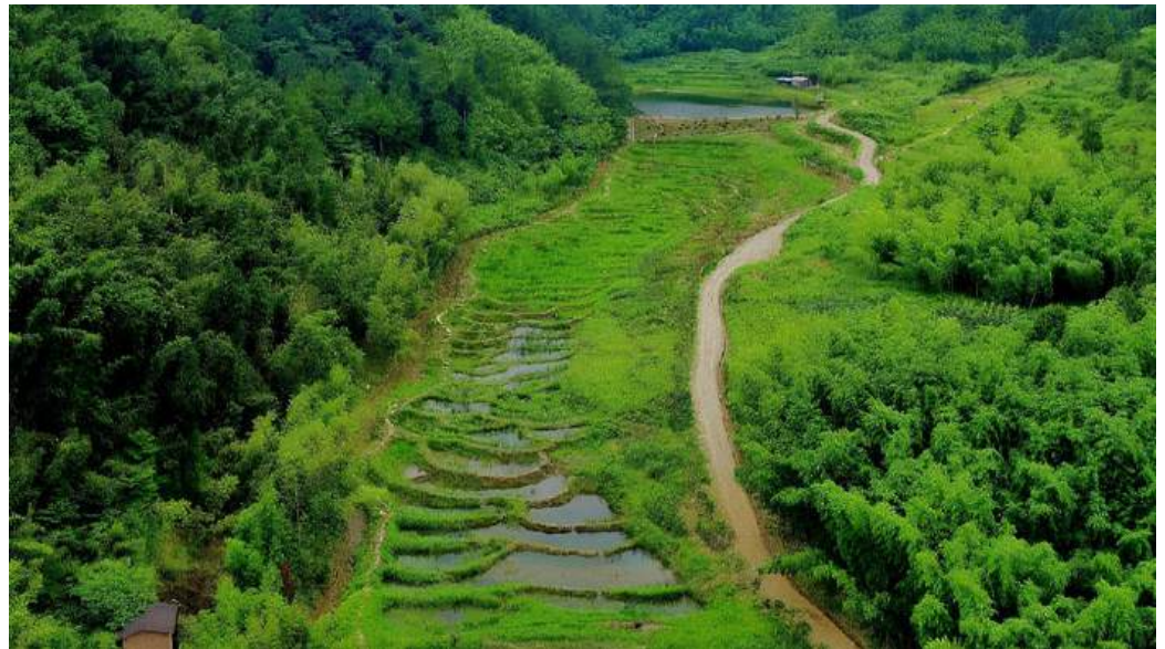
Terrace small wetlands for flood retention and pollution treatment in Liang Ping, Chongqing, Southwest China. © Lyu Cai
