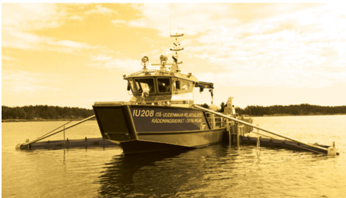
Picture 12. An oil spill collecting vessel suitable for operating in ports
