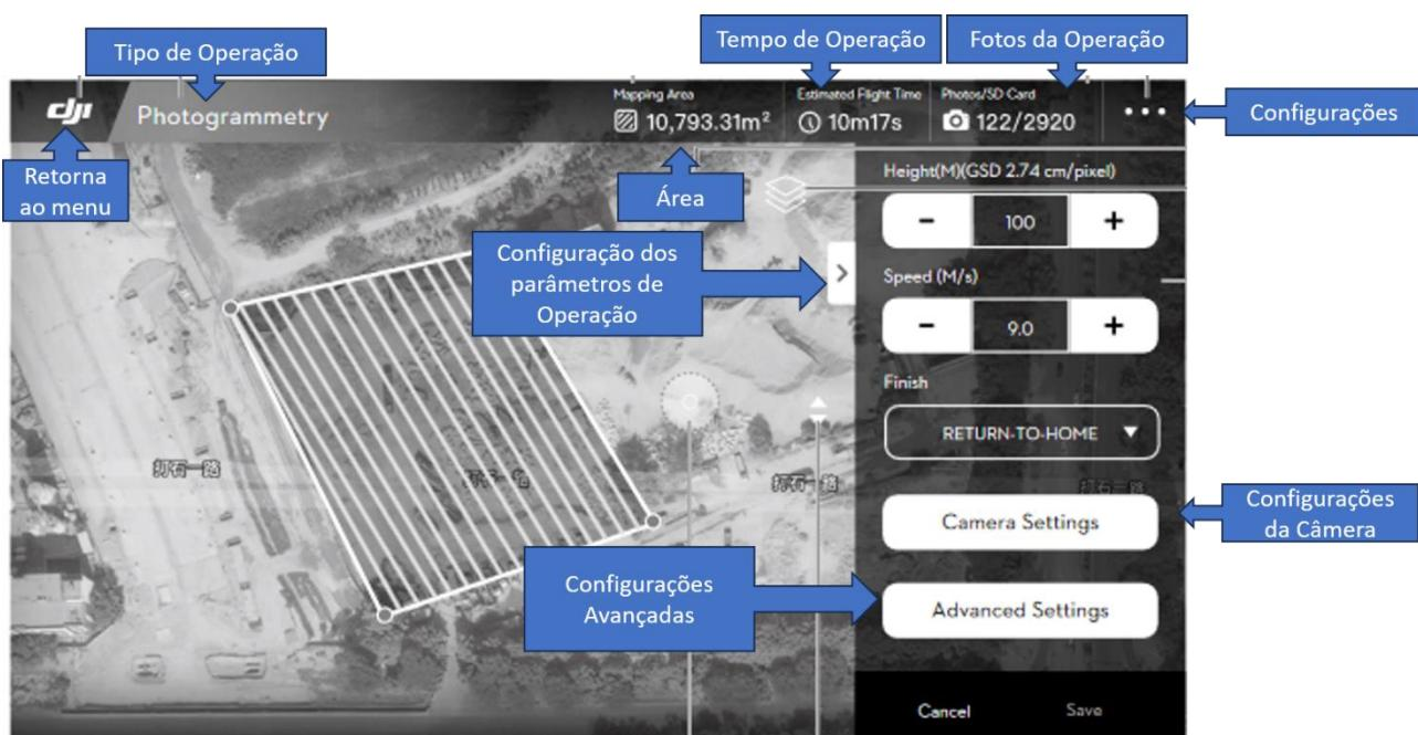
Figura 34 Tela DJI GO (modo – Plan Photogrammetry)
