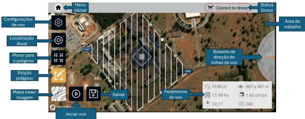
Figura 51 Interface 3DsurveyPilot
