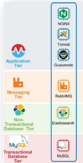
Figure 3. Single Server - Non-Redundant Combined Tiers Conceptual Diagram
