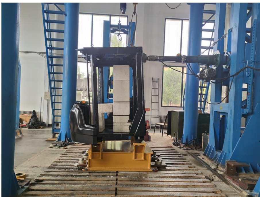
Pic. F-4 Longitudinal loading test of ROPS
