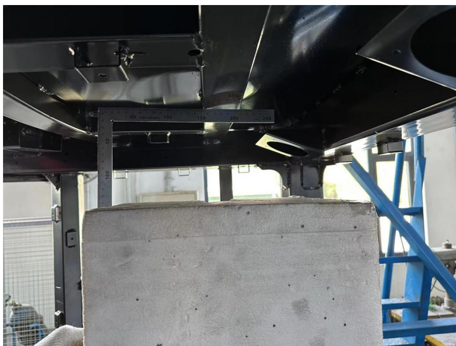
Figure D8 The relationship between FOPS and DLV after drop test
