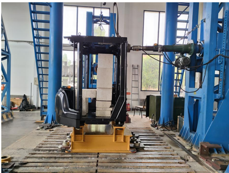
Figure D16 The loading location of longitudinal test
