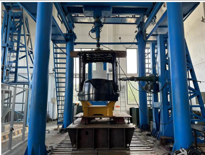
Figure D13 The loading location before vertical loading test
