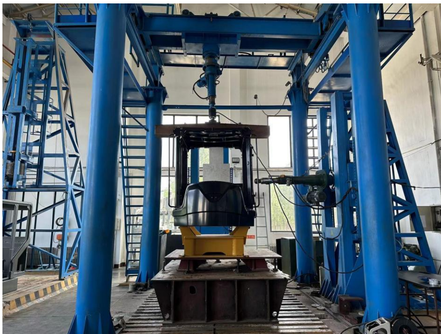
Pic. F-3 Vertical loading test of ROPS
