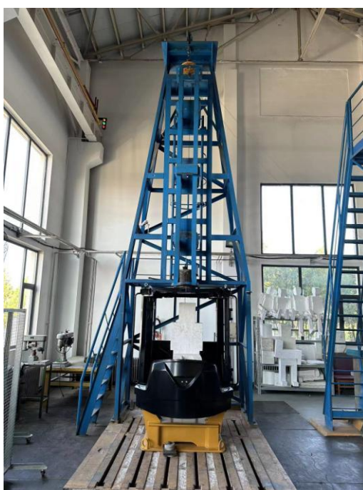
Figure D6 The FOPS fixed on the test bench after drop test
