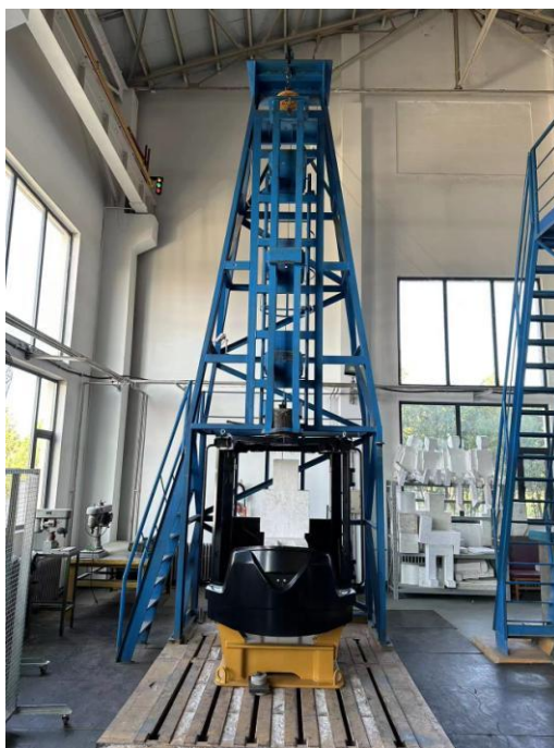
Pic. F-1 FOPS impact test
