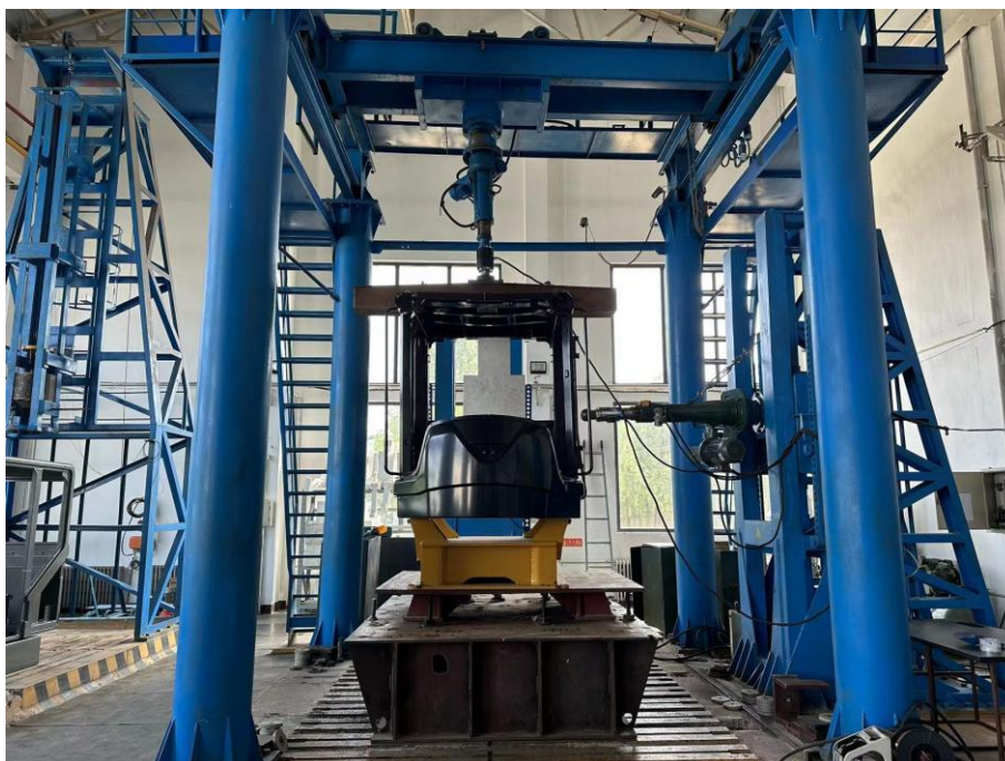
Figure D15 The vertical loading test of ROPS
