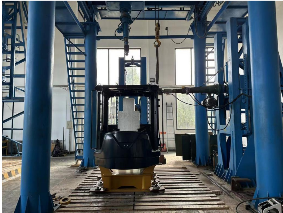
Figure D9 The location of lateral loading test of ROPS
