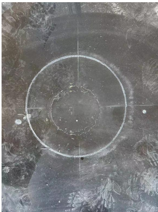
Figure D7 The deformation position of FOPS after drop test
