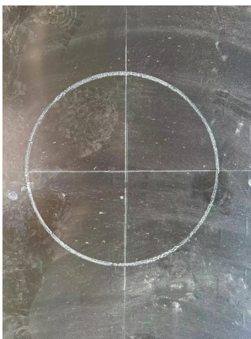
Figure D4 The falling weight point of FOPS
