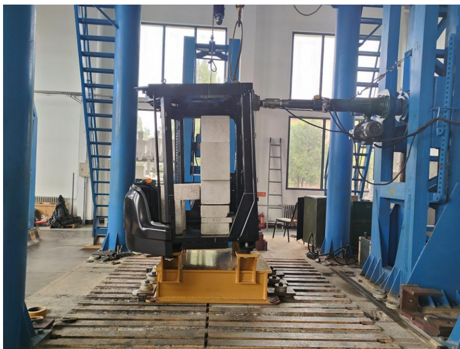
Figure D18 The longitudinal loading test of ROPS
