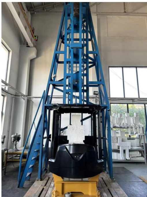
Figure D3 The FOPS fixed on the test bench before drop test
