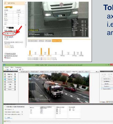
**Tolerances**: GVW: 5%, axle load: 11% i.e. 0.95 GVW and 0.89 axle load are compared to the legal limits
