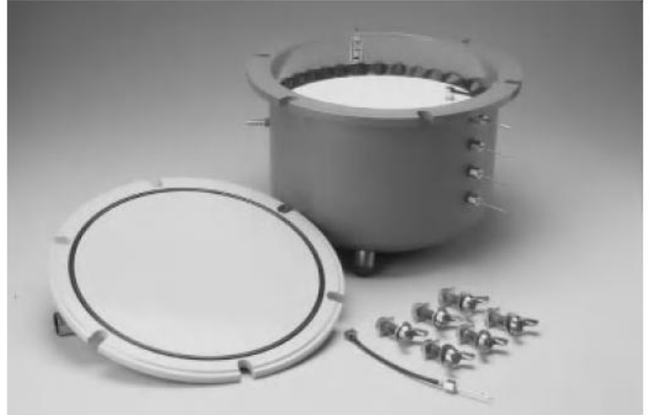
5-bar ceramic plate extractor (SoilMoisture Equipment Corporation, Santa Barbara, CA)
