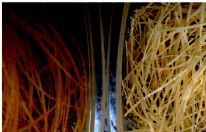
Figure 2. Samples of the propellants used in the closed vessel test: M-14 (yellow, left) and C-II (white, right).
