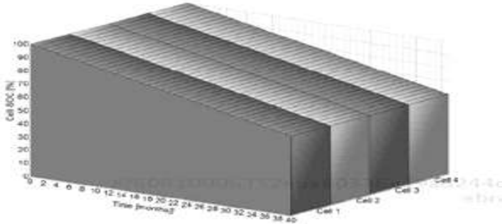
Figure 1.23 A battery on the shelf made up of identical cells. It remains balanced over time, although its SOC decreases due to leakage.
