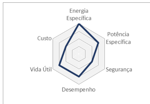
NCA - Lithium Nickel Cobalt Aluminum Oxide ( \text{LiNiCoAlO}_2 )
