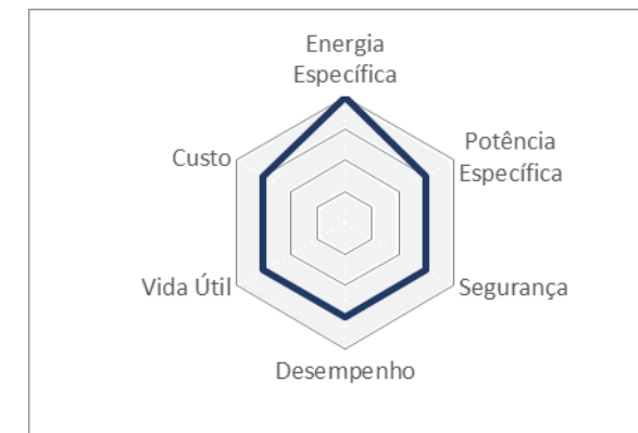
NMC - Lithium Nickel Manganese Cobalt Oxide ( \text{LiNiMnCoO}_2 )
