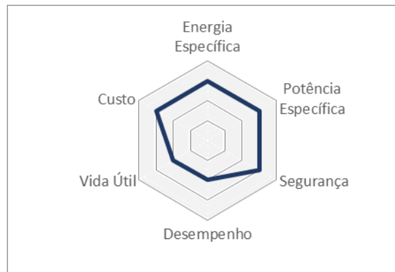
LMO - Lithium Manganese Oxide ( \text{LiMn}_2\text{O}_4 )
