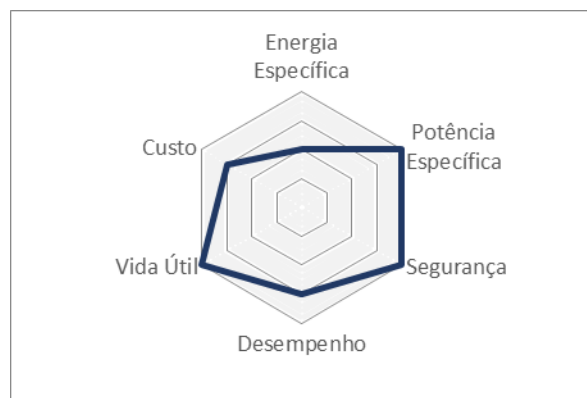
LFP - Lithium Iron Phosphate ( \text{LiFePO}_4 )
