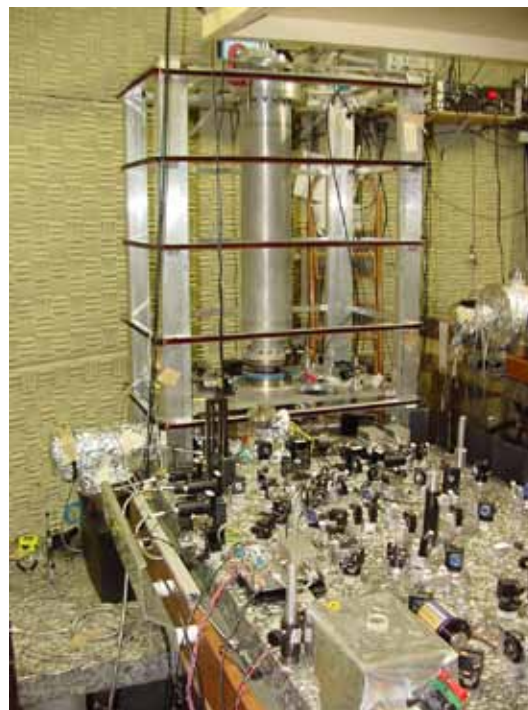
Atomic fountain clock : The most modern device for scientific time and frequency metrology
