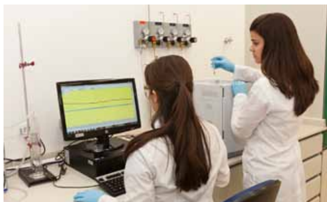
Coupled gas-chromatography-electroantennography (GC-EAG) method used to identify volatiles from plants and insect pheromones.
