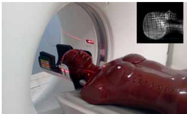
Dose assessment in anthropomorphic phantom of patients undergoing computed tomography examinations.
