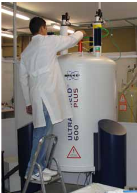
LC-NMR, LC-SPE-NMR and a 5mm cryoprobe, which will lead to an increase in the sensibility compared to a 21.1 Tesla-900 MHz for the hydrogen frequency equipment
