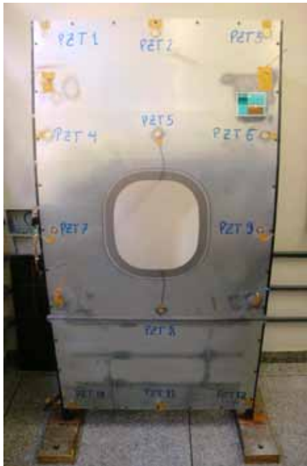
Aeronautic Panel monitored by PZT patches (health monitoring of aircraft structures)
