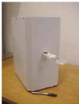
Fluorometer dedicated to the detection of luminescent markers based on rare earths ions.
