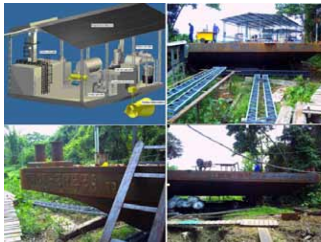
Floating hybrid system for electricity generation
