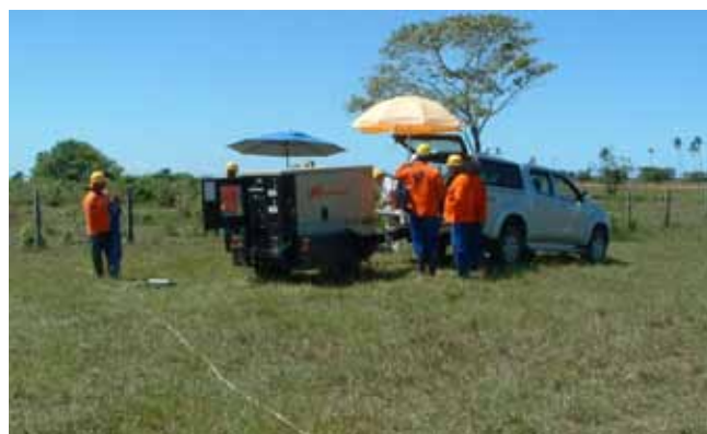
Transmission unit of the electromagnetic equipment in operation
