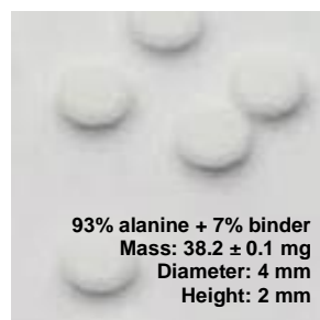
Alanine dosimeters (Aérial, France) and their respective EPR signal.
