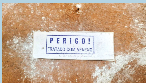
Fig. 1. Object with crystalline efflorescence and label indicating pesticide treatment from the Museu de Arqueologia e Etnologia (MAE-USP) collection.
