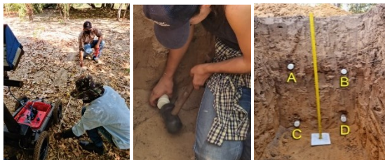
GPR scanning and trenches' sampling points. Notes: A, B at ~ 0,5 m; C, D at ~1,0 m depth.
