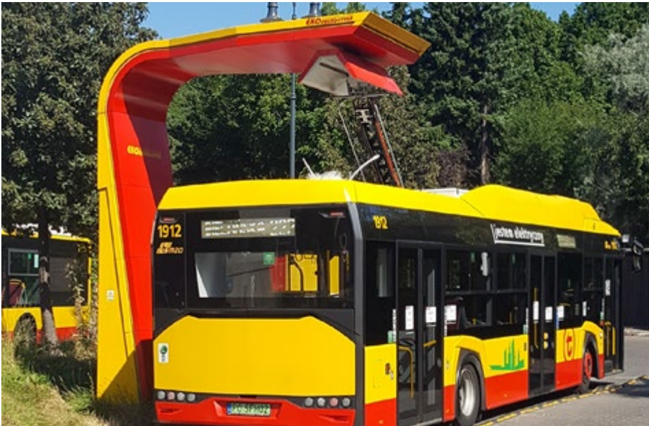
Figure 5 – Buses being charged via a pantograph in Warsaw, Poland
