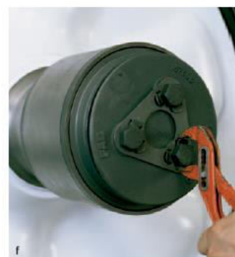
Tightening torque of the end cap screws for TAROL units with metric dimensions
