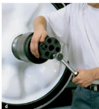
Tightening torque of the end cap screws for TAROL units with inch dimensions
