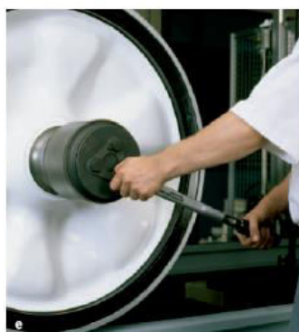
Tightening torque of the end cap screws for TAROL units with metric dimensions
