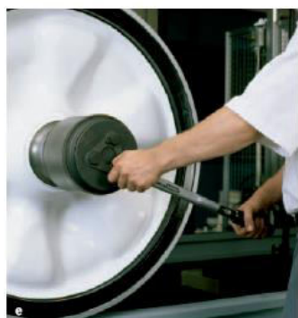
Tightening torque of the end cap screws for TAROL units with metric dimensions
