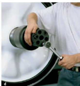
Tightening torque of the end cap screws for TAROL units with inch dimensions
