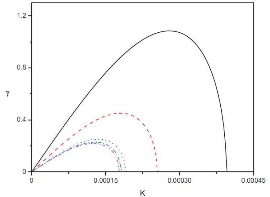
FIG. 4. (Color online)  $\gamma$  ( $\text{s}^{-1}$ ) vs  $K$  ( $\text{m}^{-1}$ ) for  $k=6 \times 10^{-3} \text{ m}^{-1}$ ,  $B_0=100$  nT and  $\kappa_e=1.8$  (solid line),  $\kappa_e=2.5$  (dashed line),  $\kappa_e=8$  (dotted line),  $\kappa_e=20$  (dot-dashed line), and  $\kappa_e=100$  (dot-dot-dashed line, Maxwellian case).
