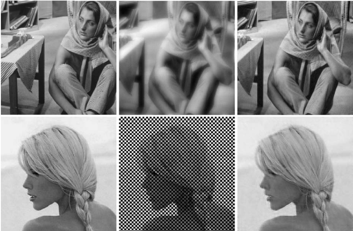
Curvelets and Ridgelets, Figure 17 Illustration of the use of curvelets (DCTG2 transform) when solving two typical linear inverse problems: deconvolution (first row), and inpainting (second row). First row: deconvolution of Barbara image, original (left), blurred and noisy (middle), restored (right). Second row: inpainting of Claudia image, original (left), masked image (middle), inpainted (right)
