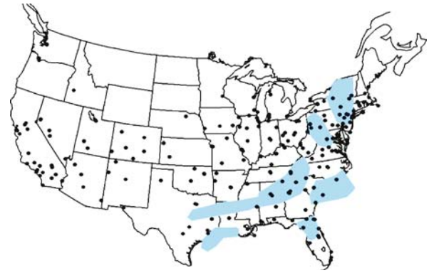
Air Traffic Control, Complex Dynamics of, Figure 10 Geographical distribution of 250G nodes in network AAN with current traffic and severe weather polygons
