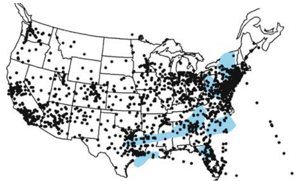
Air Traffic Control, Complex Dynamics of, Figure 13 Geographical distribution of 250G nodes in network N5 with 3X Compound traffic and severe weather polygons
