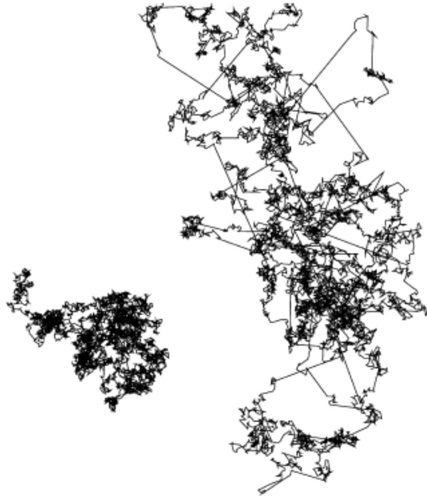
Fig. 11. Comparison of the trajectories of a Brownian or subdiffusive random walk (left) and a Lévy walk with index \mu = 1.5 (right). Whereas both trajectories are statistically self-similar, the Lévy walk trajectory possesses a fractal dimension, characterising the island structure of clusters of smaller steps, connected by a long step. Both walks are drawn for the same number of steps (approx. 7000).
