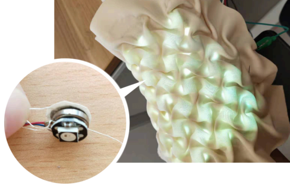
Fig. 3. The electronic components integrated with the pressure sensor, LED and vibration module, as an independent interaction unit.
