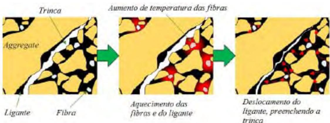
Figura modificada de GÖTHE-MEIJDE, et. al. 'Effect of different carbon nanotube asphalt self-healing via induction and infrared heating'.
