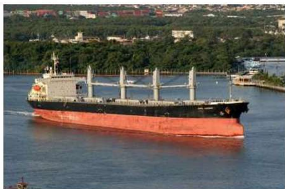
(a) Crane-based self-unloading vessel
