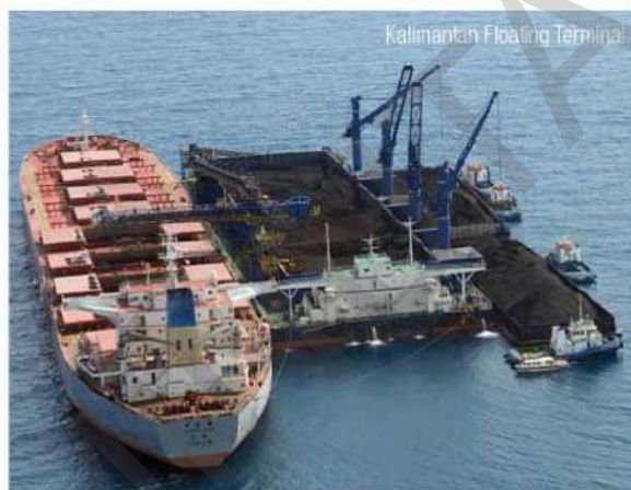
Figura 2 — Transbordo flutuante indireto [Indirect floating transshipment]
