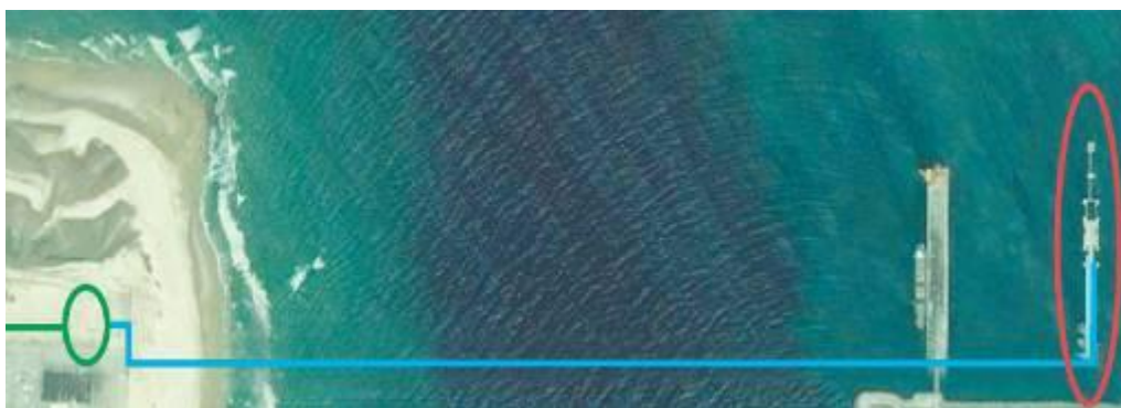
Figure VIII.7 - Layout of the gas pipeline interconnecting the Pecém LNG Pier to the MPX Filtration Station. Captions: red ellipsis: pier; blue line: air gas pipeline layout; and green ellipsis: pig launcher (Adapted from GALVÃO ENGENHARIA, 2008).
