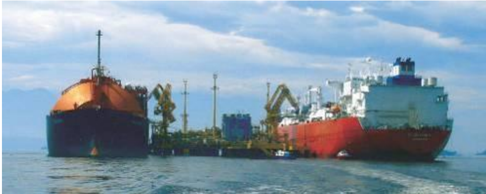
Figure VIII.1 - Panoramic view of the Guanabara Bay LNG Project, showing the re-gasifying ship Golar Spirit, to the left of the supplying vessel.
