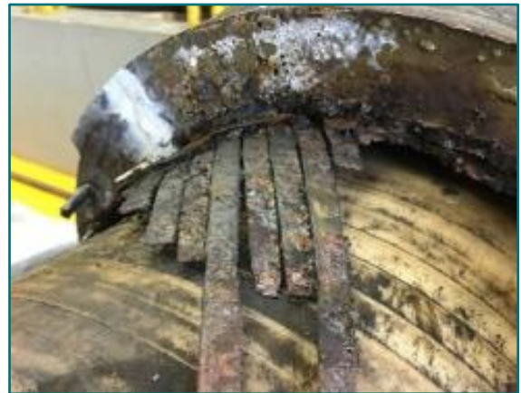
Figure 3 – Severe corrosion of the riser end fitting tensile armour wires
