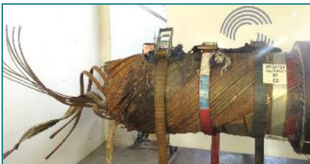
Figure 4 – Severe corrosion of the tensile armour at the end of ruptured riser section
