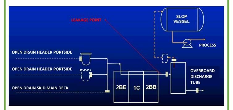
The oil stored in a cargo tank migrated into the deactivated pipe due to a hole in the empty pipe section that passes horizontally through the inside of the cargo tank, which was immersed below an approximately 1.5 m oil column when the tank was at its full capacity. The last inspection inside the cargo tank had not identified any damage to that pipe. Another hole in overboard discharge tube upstream the isolation valve allowed the leakage of oil into the sea.
