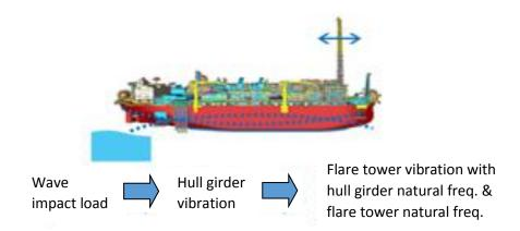
The Root Cause Analysis performed by the operator confirmed that the severe conditions and dynamic amplification due to nonlinear response (whipping effect) would lead to a flare tower structure reduced fatigue life down to couple of months.
