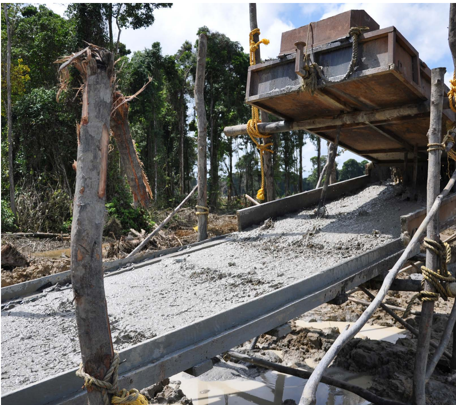
Small scale miners using a sluice box to mine for Gold in the rainforest, Guyana.
