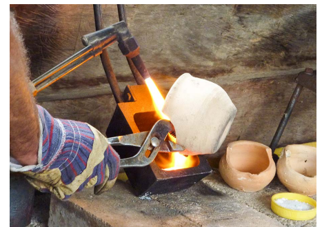
The concentrated gold charge is heated with Borax before being poured into a Gold bar, Guyana.
