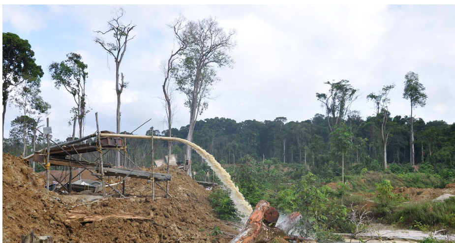
The landscape of a gold mine in the rainforest. Small scale miners using a sluice box to mine gold rich sand and clay, Ecuador.
