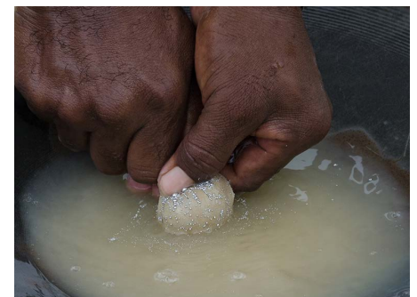
Left: Men gold panning in shallow river, Masango, Cibitoke, Burundi. Below: Miner uses mercury to separate out the gold from waste minerals, Guyana.
