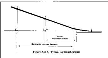
The airplane reference point for approach measurements is the instrument landing system (ILS) antenna. If no ILS antenna is installed an alternative reference point must be approved by the FAA.
