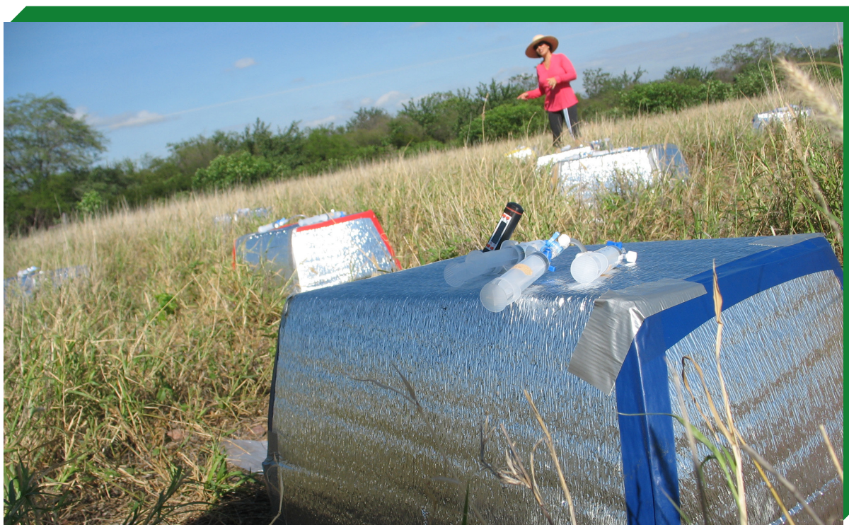
Figure: Chamber for monitoring greenhouse gas emissions in the soil in an area of Buffelgrass.
