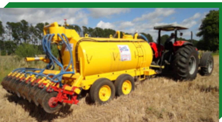
Figure: Equipment developed for the injection of liquid animal waste into the soil in no-till system
