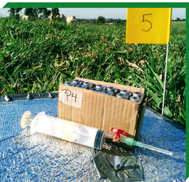
Figure: Static chambers used to collect N 2 O used in the study.
