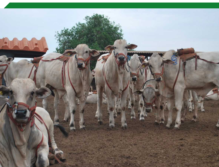
Figure: Collection of individual methane emissions from cattle confined in a collective stall. Sulfur hexafluoride tracer gas technique.
