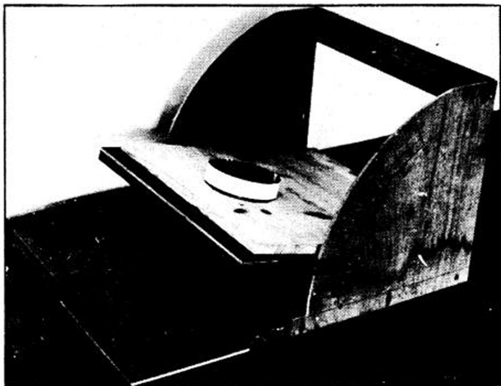
Figure 1 - Tilting table used for coefficient of friction studies of cocoa beans at various stages of drying.
